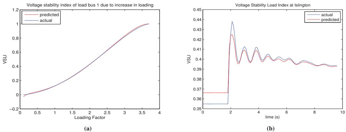
**Figure 5:** (a) Voltage stability load index variation at Invercargill as a result of increased loading at Invercargill. Load is increased from base load to the point of voltage collapse. (b) VSLI variation at Islington due to 25% increase in real power loading from base case.
