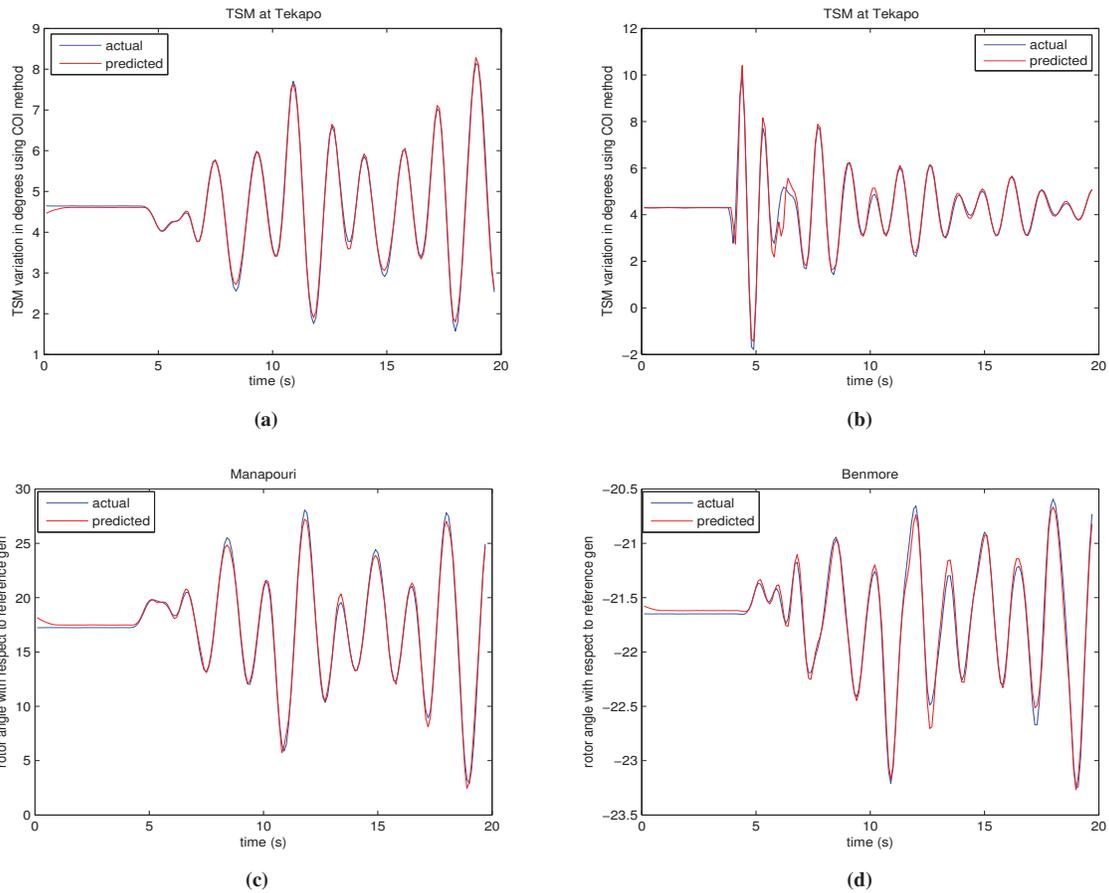
**Figure 4:** (a) Transient stability margin of generator at Tekapo when subjected to PRBS injections. (b) TSM variation at Tekapo due to 6-cycle three phase to ground fault at Islington. (c) Rotor angle deviation prediction for generator at Manapouri when subjected to PRBS injection. (d) Rotor angle deviation prediction for generator at Benmore when subjected to PRBS injection.
