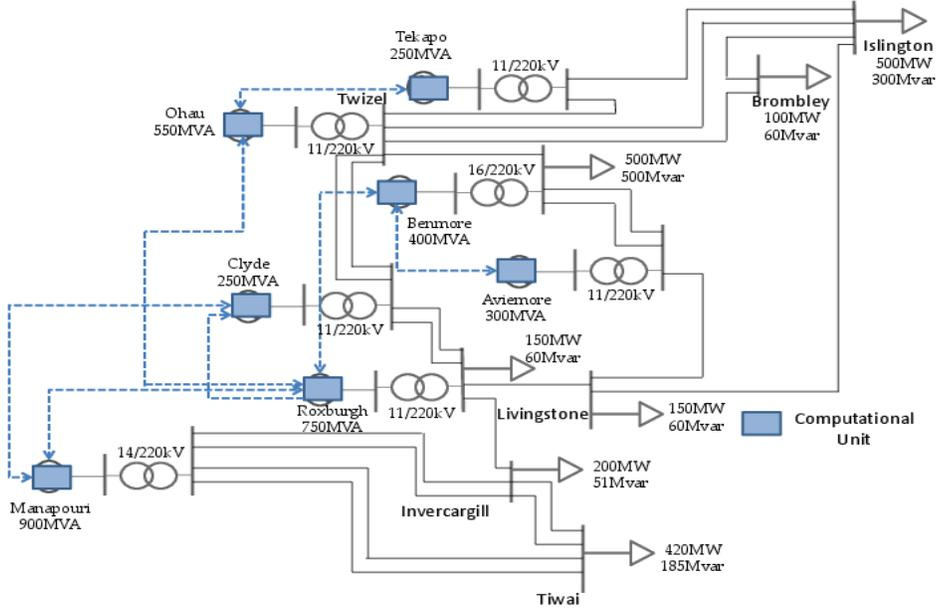
**Figure 2:** Transient stability margin prediction scheme is shown. Computational units are superimposed on top of one line diagram to show how spatial dynamics are captured. Information exchange is shown as directed arrows.
