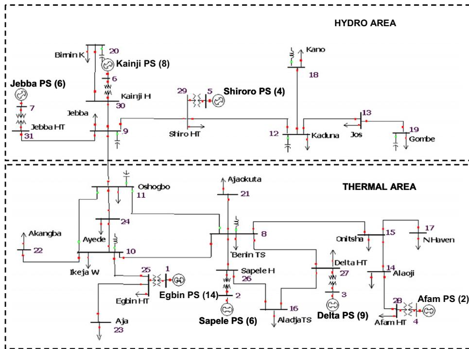
Fig. 3. Nigerian 330 kV grid showing seven power generating stations.
