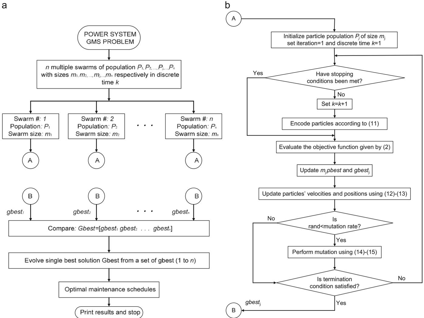
Fig. 1. MS-MDPSO algorithm framework for power system GMS problem: (a) *n* multiple swarms-MDPSO and (b) MDPSO implementation for multiple swarms application.
