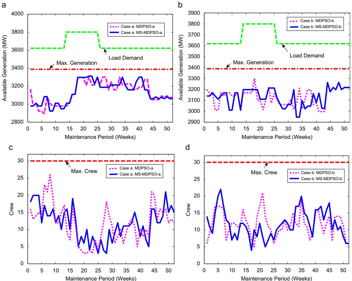
Fig. 4. Generation and crew plots during maintenance period: (a) available generation versus maintenance period for case a: MDPSO-a and MS-MDPSO-a, (b) available generation versus maintenance period for case b: MDPSO-b and MS-MDPSO-b, (c) crew requirement versus maintenance period for case a: MDPSO-a and MS-MDPSO-a and (d) crew requirement versus maintenance period for case b: MDPSO-b and MS-MDPSO-b.
